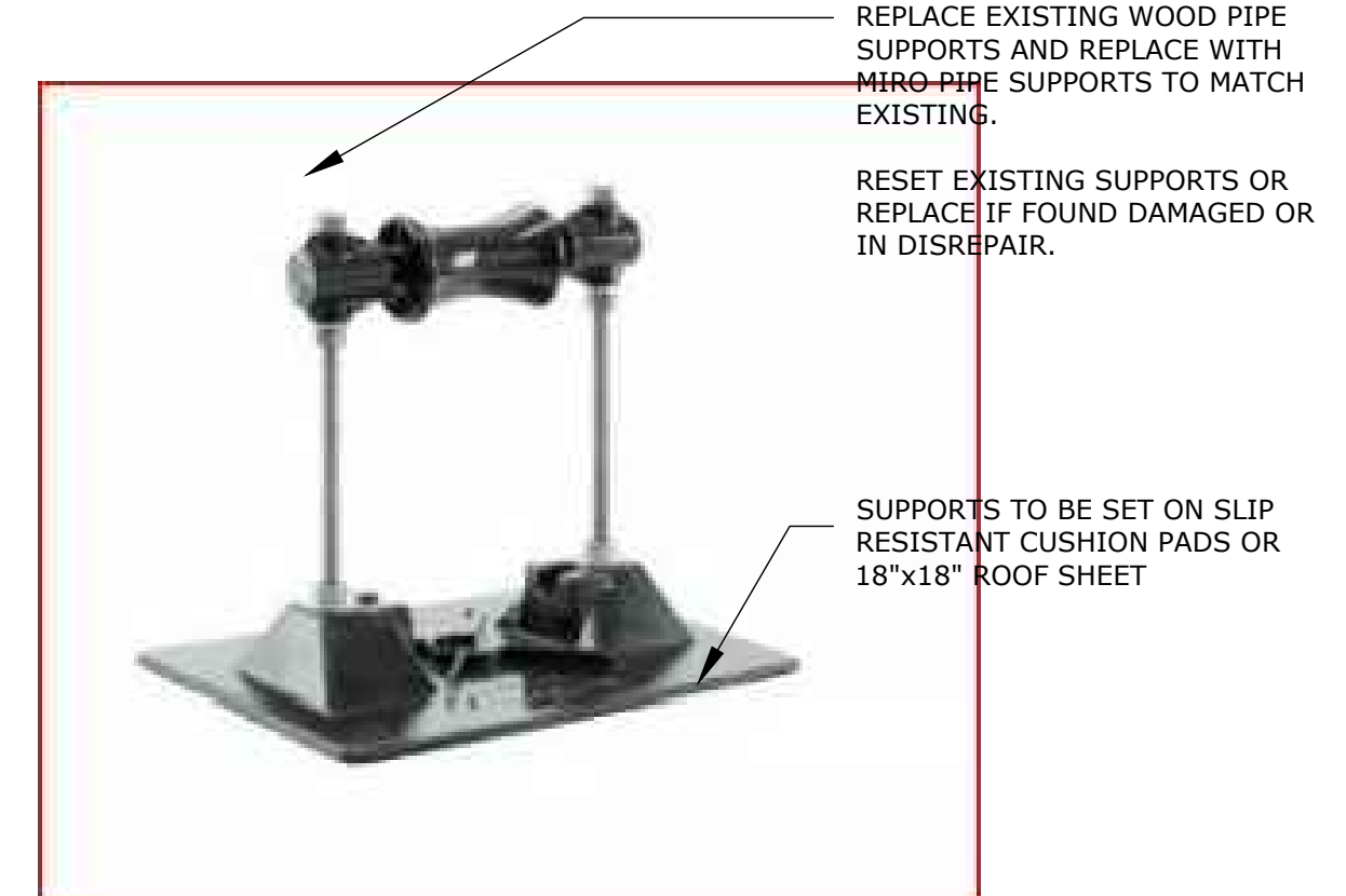
4 PIPE SUPPORT DETAIL SCALE: 1-1/2" = 1'-0"
